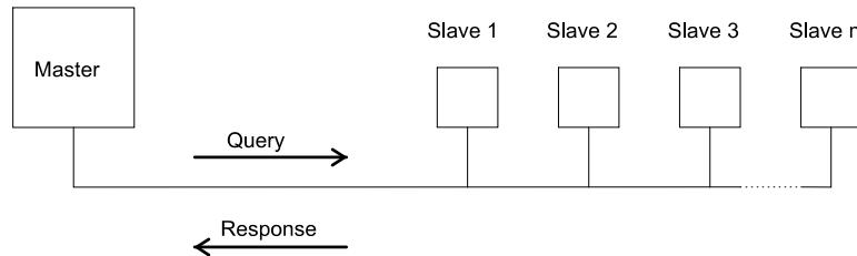
In the MODBUS™ Protocol the master can address individual slaves, or, using a special “Broadcast” address, can initiate a broadcast message to all slaves. The Integra, INT-2100 digital power quality meter does not support the broadcast address.
