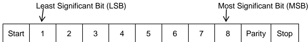
Transmit Character = Start Bit + Data Byte + 2 Stop Bits (11 bits total):
